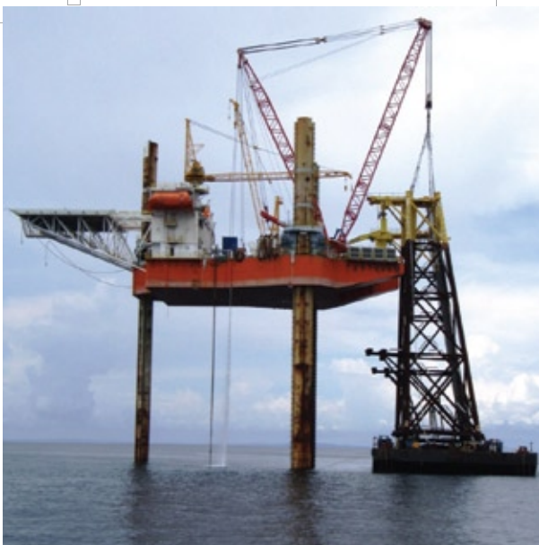
2007 - A 1,200 te capacity crane mounted on an Al Jaber jack up barge in Malaysia
