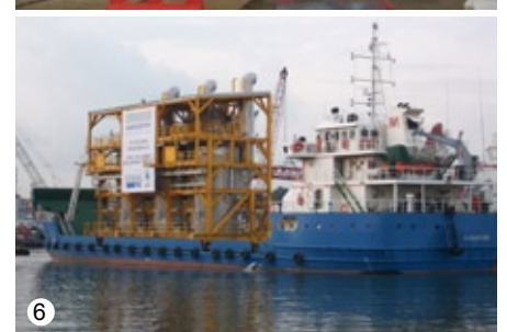
1 to 6 above – Fabrication, overland transport, lifting and marine transport of an LP Boiler module by AOS at their waterfront facility in Singapore.
