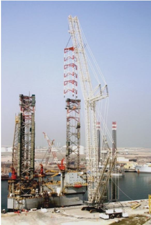
3,200te capacity Demag CC8800-1 with a crawler twin attachment in the Middle East lifting 425te at 60m radius with 200m of boom.
