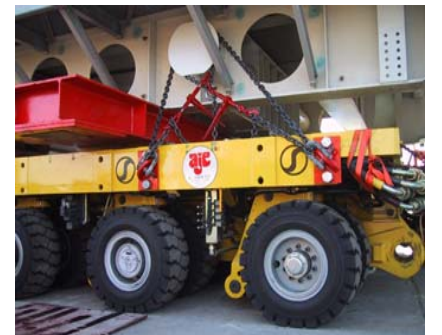
Our site supervision executes quality checks of lashing and stability prior to transportation of the load
