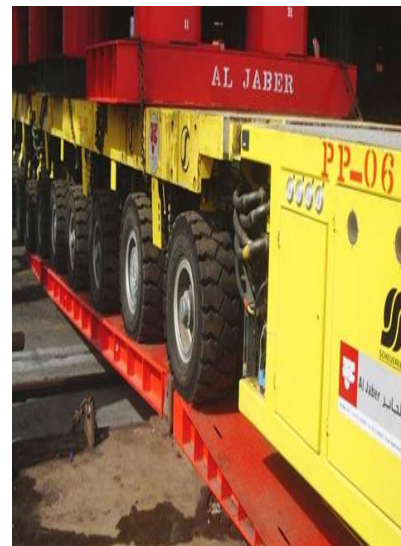
Modular Trailers with capacities upto 40 te per axle line.
