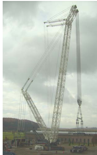
Cranes up to 3200 te capacity.
