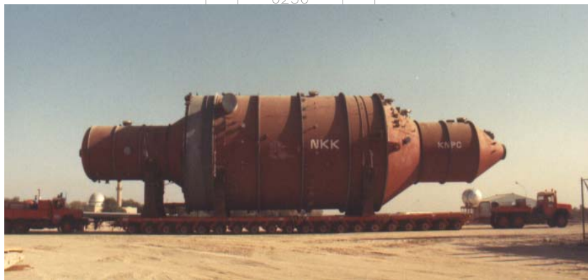
1984-Transporting a 370 te reactor in the U.A.E
