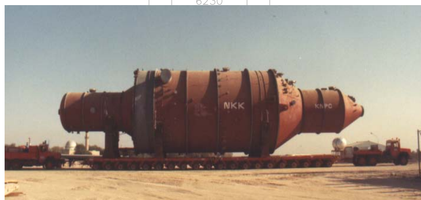
1984-Transporting a 370 te reactor in the U.A.E
