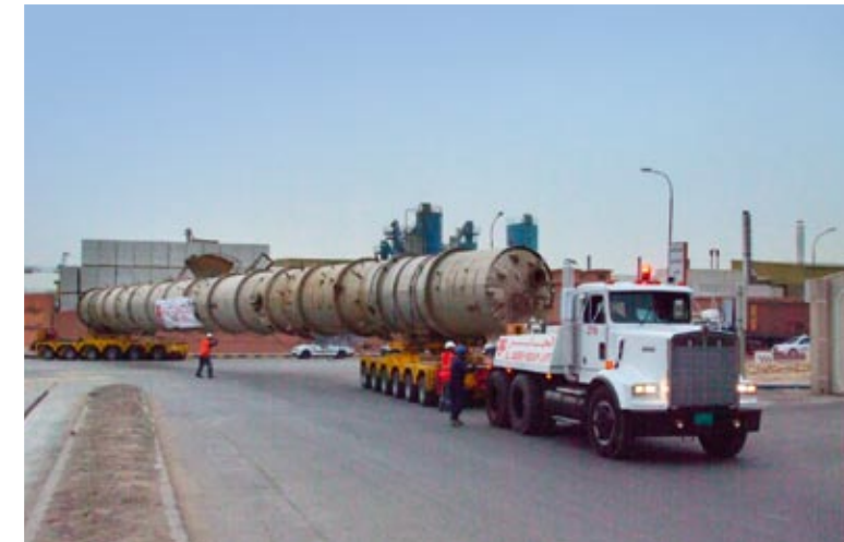
△ Transportation of a 43 meter long vessel using 24 axles of conventional hydraulic trailers in the Kingdom of Saudi Arabia.
