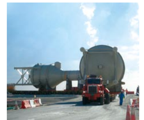
△ Transportation of a 240 te brine evaporator utilising 24 axles of conventional hydraulic trailers in Qatar.
